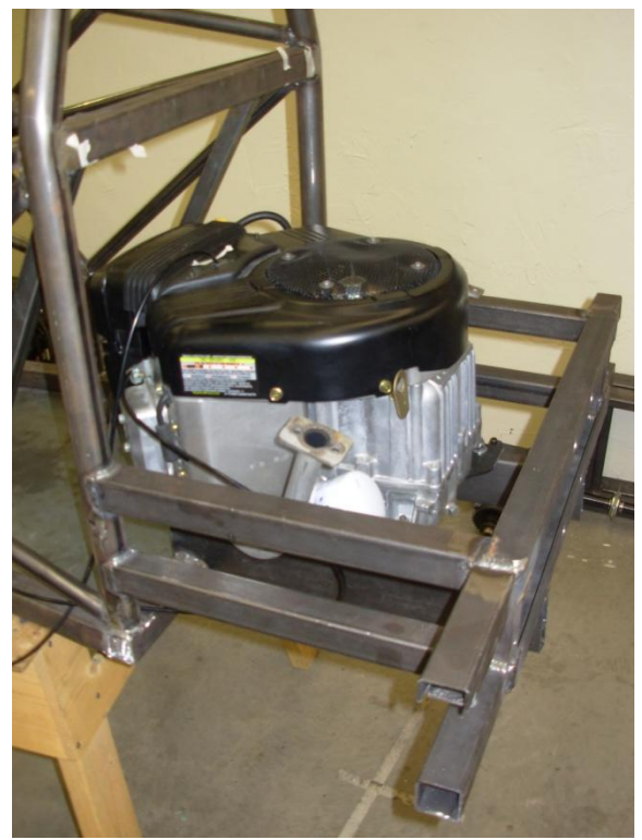
Back end with engine mounted. The rear axle is almost done.
