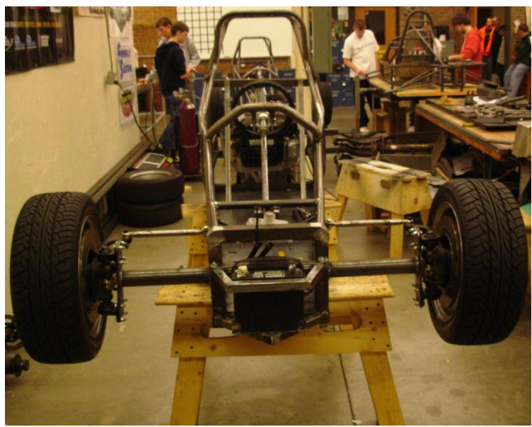
Chassis with the front axle complete with battery in front for added traction.
